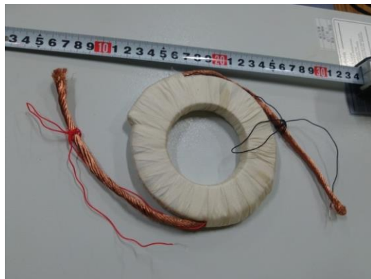
Fig. 4. Photograph of the coil after epoxy solidification. Outside of the coil was wrapped with silk tape for protection.
